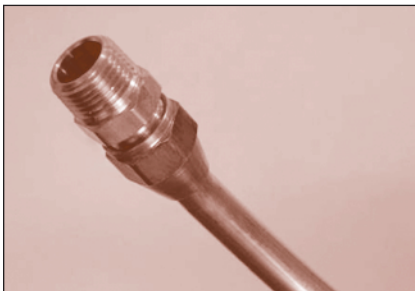
FIGURE 29: Completed Flared Joint
