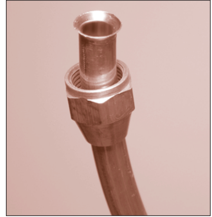
FIGURE 32: Completed Flared Tube End
