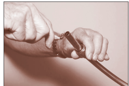
FIGURE 30: Reaming Prior to Flaring the Tube End
